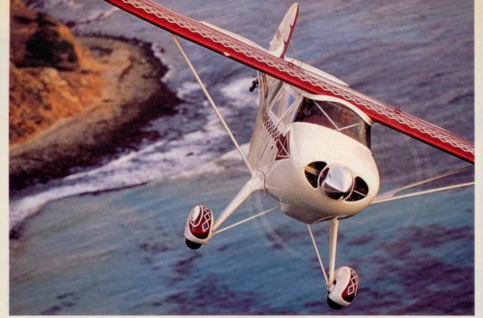
work load is higher during taxi, takeoff, and landing than with tricycle-gear aircraft. While the cowling has been lowered three inches, forward visibility remains greatly reduced during taxi. A takeoff run of only a few seconds was required before the tail could be raised to provide a view of the runway ahead.
