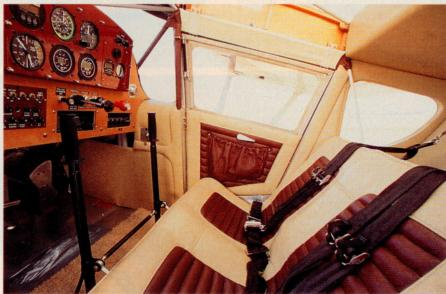
Even with the lowered cowling, the view out of the front is limited on the ground. Four-point harnesses hint at the 110's aerobatic capabilities (above).
